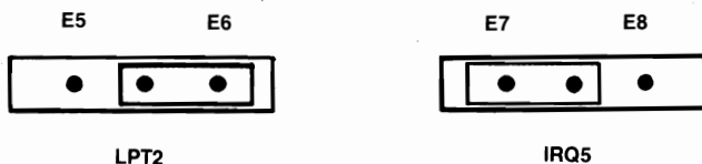
Figure 3-6. Parallel Port Configuration with Another Video Display Card with a Built-in Printer Port (PC-AT).
