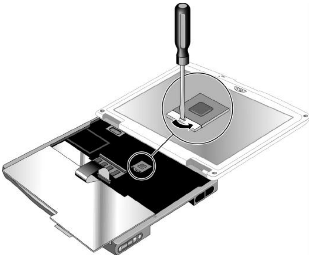
Figure 2-19. Removing the CPU Module
