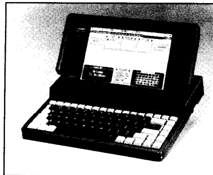
The Tandy 1500 HD comes with a standard 3.5-inch floppy drive and a 20 MHz hard drive.
