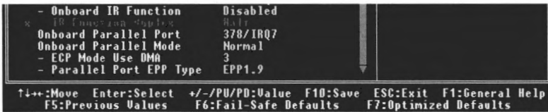
Figure 3-6D. Integrated Peripherals Menu Full Items Screen (KT7-RAID)
