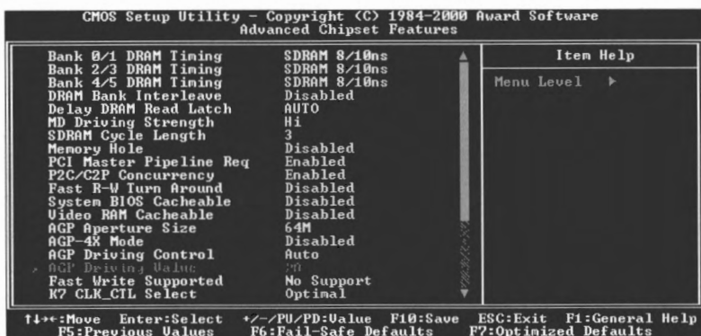
Figure 3-5A. Advanced Chipset Features Setup Upper Screen
