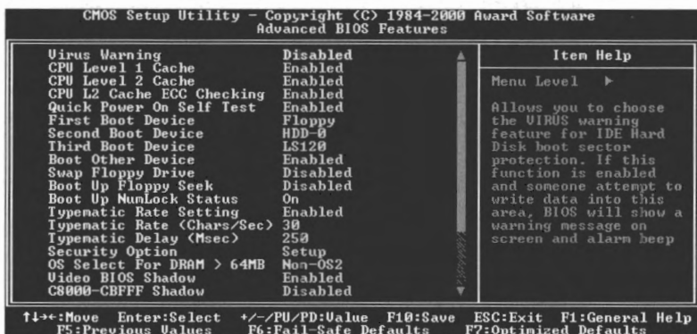
Figure 3-4A. Advanced BIOS Features Setup Upper Screen
