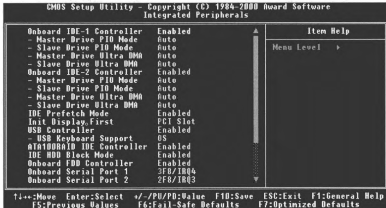
Figure 3-6C. Integrated Peripherals Menu Default Screen (KT7-RAID)
