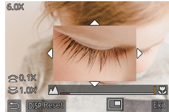
Focus with AF, then fine tune with MF after AF locking. Confirmation is possible while enlarging with MF Assist.
