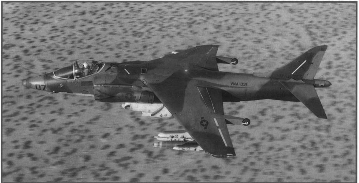
An AV-8B of VMA-331 'Bumblebees' flies over the desert carrying 500 lb 'Snakeye' retarded bombs.
