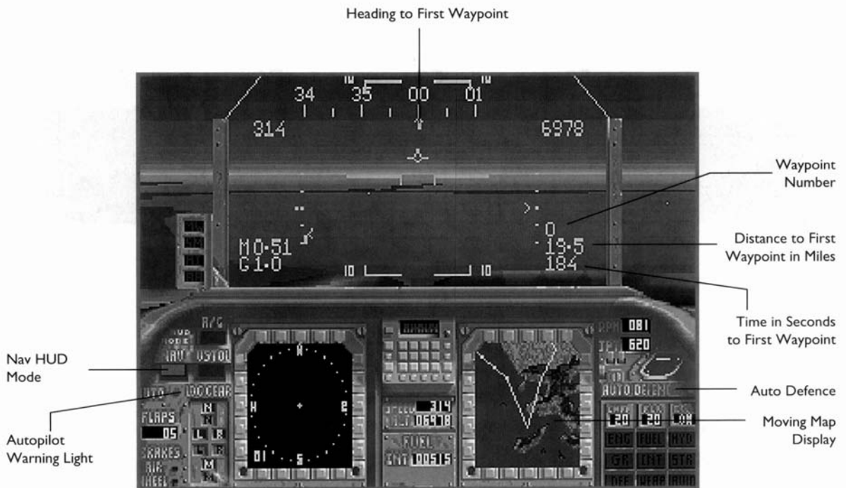
The Harrier Cockpit in Nav HUD Mode
