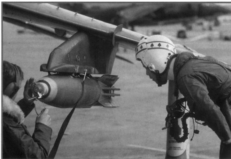
A pilot checks the arming of a MK.82 Snakeye bomb on his Harrier
