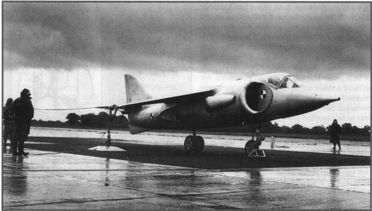
The prototype P.1127 during a tethered hover test.
