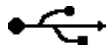
Figure 1: The USB symbol found on the Pro Pedals USB plug and the USB connector on your computer.
