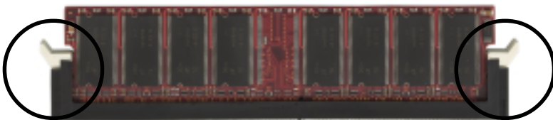
Figure 9 - DIMM module clip after installation
