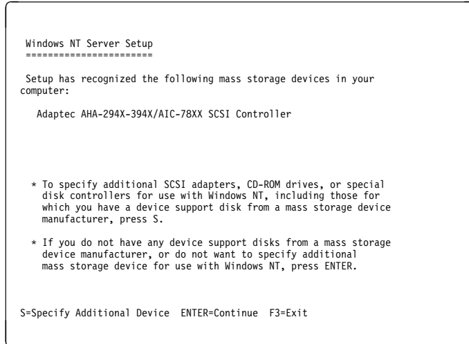
Figure 56. Disk Controllers Detected During Installation. This panel applies to the PC Servers 325, 330 and 704; other servers are similar.
