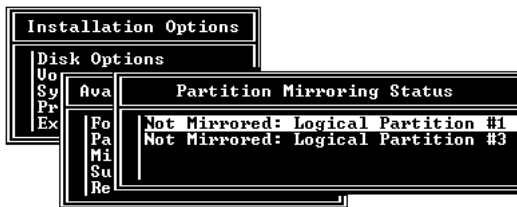
Figure 2.13 Partition Mirroring Status Screen
